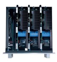
Modular design with independent power supplies each with its own transformer for precise sound-staging.
