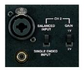
Input flexibility: XLR or 1/4" phone jack for balanced signals and RCA jack for single-ended source; input gain is selectable.
