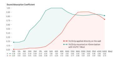
NRC: VicStrip applied directly on the wall: 0.45; VicStrip mounted on 45mm batten with VicPET Wool (40mm) behind the panels: 0.85.
