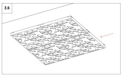
Please note: It should be applied a blocking element such as a L profile to avoid the last panels to slide off the VicFix J profile. Vicoustic will not take responsibility for any mistakes/ limitations occurring during installations or any damages resulting from falling panels.
