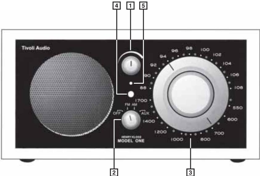
1. **VOLUME KNOB:** Rotate the volume knob to the right to increase the volume or to the left to decrease the volume. This knob also controls the volume of the headphone output.
