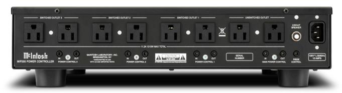
Designed to accommodate various global power standards, the MIP200 is available with either 4 Type B (NEMA 5-15R) outlets with 2 receptacles each (above), or 4 Type F (CEE 7/3 or "Schuko") outlets with 1 receptacle each (below).
