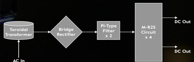
*Note: There are 2 circuits like this block diagram in the 820S; one each for the analog and digital power supplies.*
