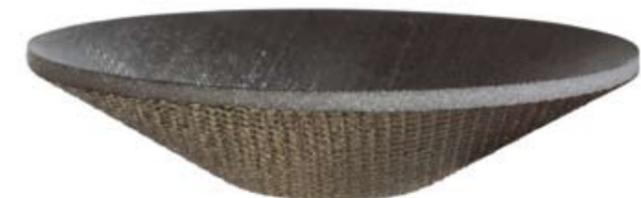
Bass cones must be as light as possible for maximum agility, but absolutely rigid in order to retain their shape as they pump in and out. Rohacell® is a sophisticated composite construction made of a hard foam core sandwiched between carbon fibre skins. It's the kind of material normally used for aircraft, rockets and the bodies of racing cars. For speed, stiffness and unshakable bass, it's the bottom line.
