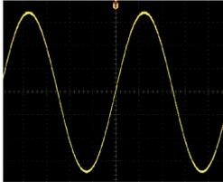
Photo (c) PS-530 output waveform (distortion approx. 0.06%)
