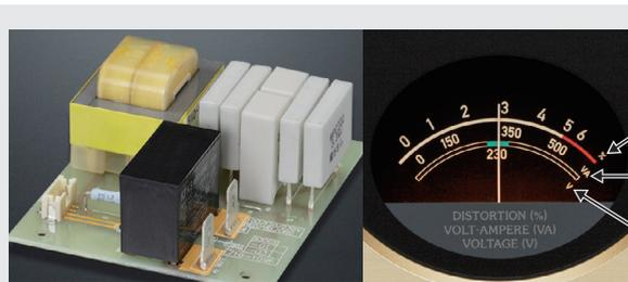
Assembly with input voltage/distortion monitoring circuitry
